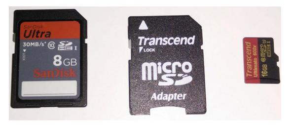
Figure 1-4. SD card with micro SD and adapter
