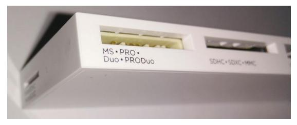
Figure 1-5. Multicard reader (micro SD reader is on the left edge near the bottom)
