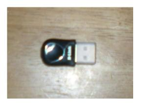
Figure 9-3. D-Link DWA-131 802.11n wireless N nano adapter
