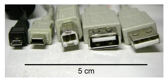
Figure 1-3. Different types of USB connectors
