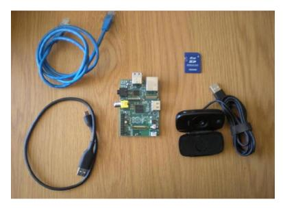
Figure 10-1. The Raspberry sPi kit
